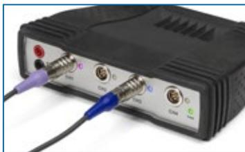
Colour guide in software and hardware guides the user through automatic sensor recognition.
