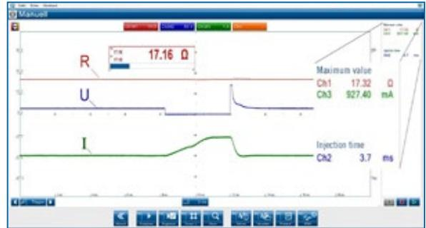
Simultaneously measure resistance (curve and nominal value), voltage curve and current curve for injection valves.
